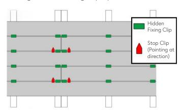
Only one stop is to be used per board, creating a maximum of one butt join per run of decking. The screw going into the decking board must be predrilled.
