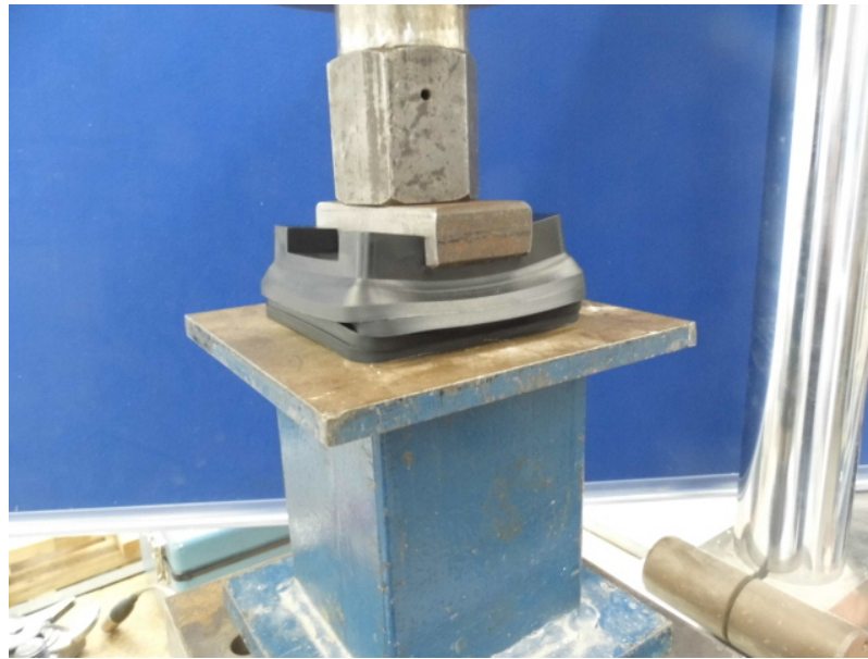
Figure 6. Failure of Joist Mount with Three 3 mm Thick Packers during Compression Testing
