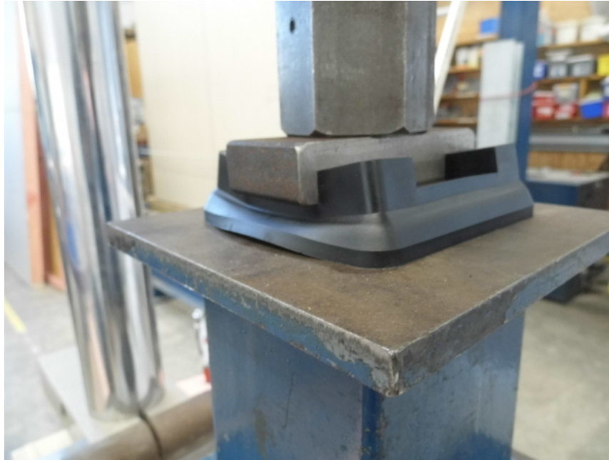
Figure 4. Failure of Joist Mount during Compression Testing
