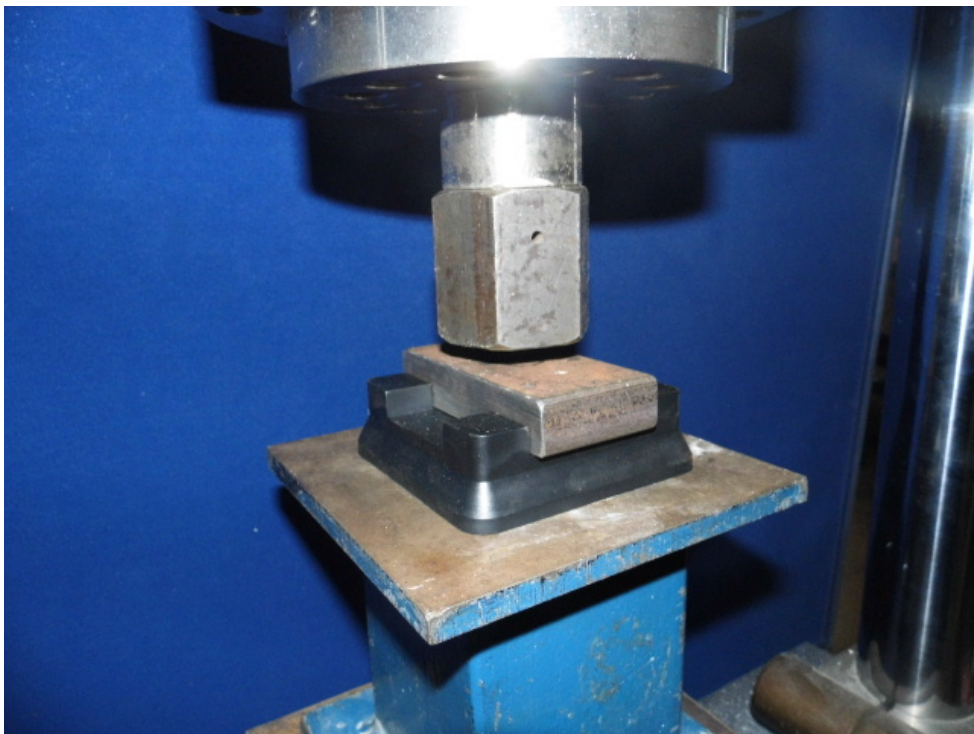
Figure 3. Testing Set Up for Biform Joist Mount and Packer Testing (Only Joist Mount Shown Here)
